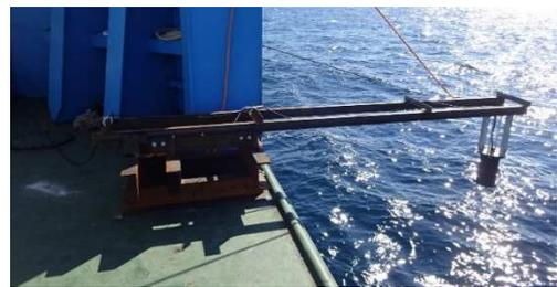
Fig. 10 Microwave type wave height meter
