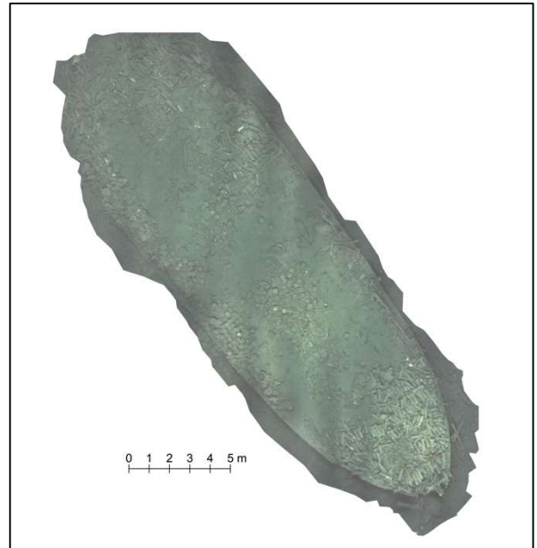
Fig. 10 Ortho-mosaic image with 1m interval of survey lines using high accuracy of alignment of images
